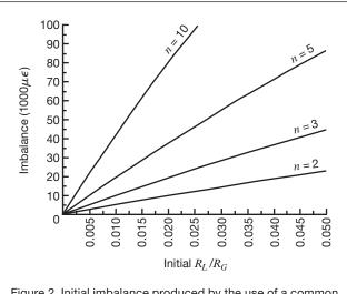
**Errors Due to Shared Leadwires in Parallel Strain Gage Circuits**
